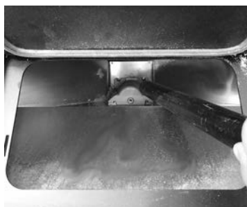
Fig. 33 - Hopper and auger cleaning
